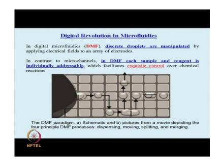
Now, this is an interesting picture which where I would like to spend some time, now we would like to see how discrete droplets can be manipulated by electro by electric fields to an array of electrodes.
