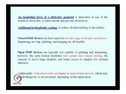
So, there are certain advantages to this closed format of DMF and the open format of DMF and we would see what they are. Now this I have already described is the importance of the insulating layer, importance of the hydrophobic coating and so on. The close DMF devices are very well suited for a number of droplet operations, you can move droplet, you can split the droplet into two and even you can merge two droplets to to make one large droplet.
