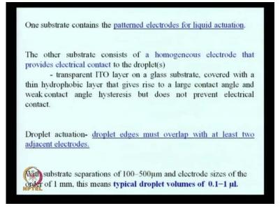
So, I will move on to the next is the substrates that are used it could be a transparent glass with ITO coated having a thin the hydrophobic layer. And the droplet edges must overlap with at least two adjacent electrodes, in order to have any kind of actuation. And the typical droplet volumes which are encounter are encountered in this or these operations are between point one to 1 micron per liter 1 micro liter.
