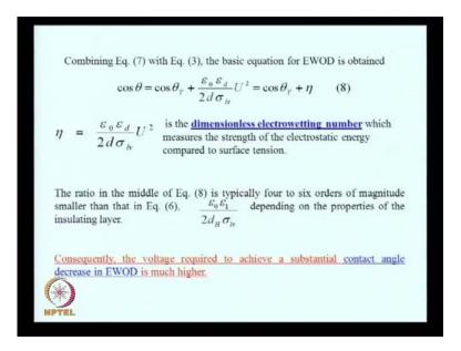
And finally, incorporating the concept of electrowetting the following equation has been has been derived has been, we have seen this class, where cos theta is the angle cos theta is the angle it is essentially the contact angle on application of voltage. Theta Y is the contact angle at equilibrium contact angle without any voltage and U is the applied voltage, sigma is the surface tension, d is the thickness and so on.
