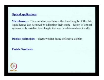
The in the optical applications, I would the only spend I will I will only say few words about the micro lenses, because if you if you could create a lens using a droplet a liquid droplet the advantage is that it is very flexible and by applying the right electric field, the
