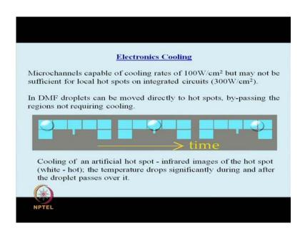
And if I would like to use the droplet for electronics cooling, you would see that this is the droplet, this is a hotspot the whiteness shows the hotspot. And as the droplet moves comes to this point, the hotspot disappears as the droplet moves away from it you would see a faint reappearance of the hotspot.
