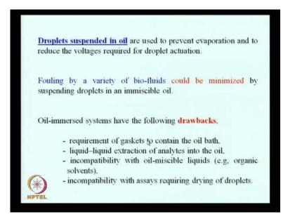
In some cases specially in closed digital micro fluidic systems, the droplets are suspended in oil they they have suspension in oil does are fulfills two purposes. One is it does not allow any evaporation to take place and the second is there are certain bio fluids, which which corrode the surface or which which deposits on the surface and it is difficult to clean such a surface.
