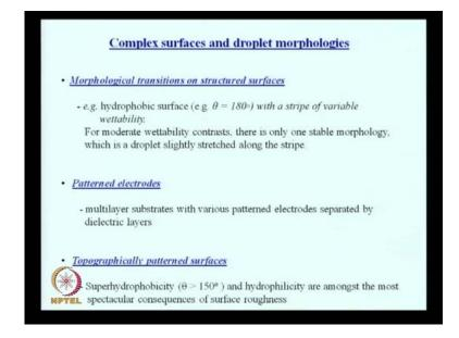
So, we are now going to we will with this background we are going to start our this class with complex surfaces and droplet morphologies, how the complex surfaces would give rise to motion in the droplet. So, we know that hydrophobics there are there are cases where hydrophobic surfaces with a strip of variable wettability can be used to move a droplet. So, let us say we have a surface in which the hydrophobicity keeps on changing.
