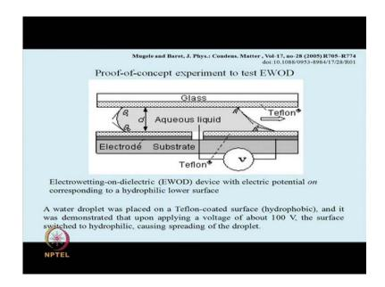
Now this is a proof of concept experiment to test how EWOD works, now here you see that we have an electrode electrode electrode and then this is the dielectric and we have thin hydrophobic coating on the surface; such that the electrode the such that the droplet or the plug as is as in this case can move easily with less amount of contact angle hysteresis.
