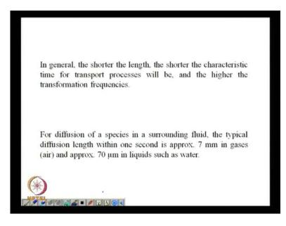
So, summary we can say that the shorter the length, the shorter is a characteristic time for the transport process and the transformation frequency is going to be higher. And just to give you an idea that what we are talking about in terms of diffusion length, is roughly about 7 millimetre in gases and approximately seventy micronin liquids. That is the diffusion length length covered by a diffusing molecule in a second.
