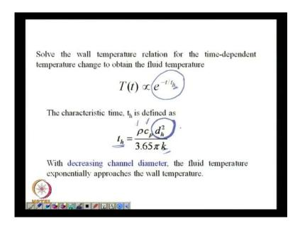
So, the temperature isgoing to exponentially change with the distance traversed and when we connect this characteristic length with the velocity and so on then this t x, the temperature change in temperature can be related to an exponential change with time andwe could see that the characteristic time which ishere in the denominator is it can be connected with rho, the density, c p the pthe heat capacity thermal conductivity but, most importantly with the square of the size of the device.
