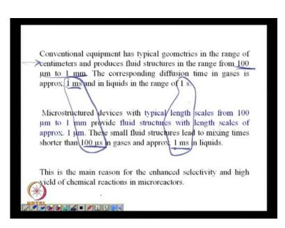
Now when we think of a macro device a macro device has a length scale which is typically in the range of centimetres. In in this fluid packets with with which you can represent the thethe process in a conventional equipment their sizes are for from 100 micron to about 1 millimetres and a corresponding, if you look at the corresponding diffusion time over here.So, we are we for micro devices we are we are working in this
