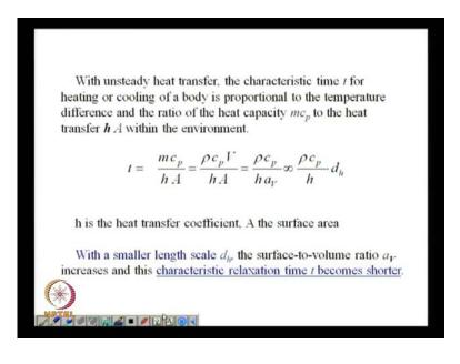
And this again is tells us something about the timenecessary for the time scale involved in unsteady state heat transfer processes. So, a smaller length scale the characteristic reduction relaxation time also becomes shorterand we will have an faster reaction taking place. The system is going to reach steady state at a much, at a value which issmaller than that of a macro system.
