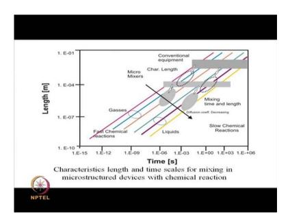
Now, over here we have the length n k l o in on  $\frac{1}{2}$  on the axis we have the time. So, it is basically a characteristic length and time scales for mixing in small devices.
