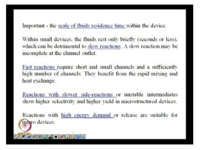
Another important thing one has to keep in mind is what is the scale of the fluid residence time inside such a deviceand within what we know is at within small devices the fluids are going to rest only for a very short time inside the reactor. So, if you have a slow reaction a micro device may not be the ideal option available for you because the residence being small the reaction may not be complete at the exit of the micro device.
