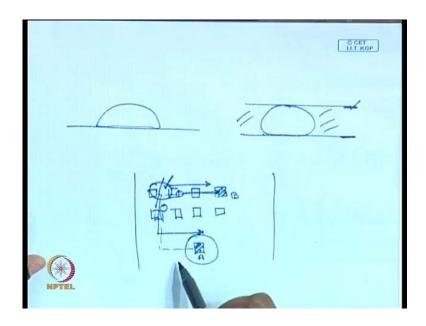
how you switch these off and on?A droplet sitting over here can be made to move either in direction or it can take any path it wants. I mean, you can program the switching on and off these electrodes and thereby, make the droplet move on any prescribed path.Therefore thereby, creating enough flexibility in the entire design of the process such that it can be split and one droplet will move in this direction, and the other droplet will move in another direction.
