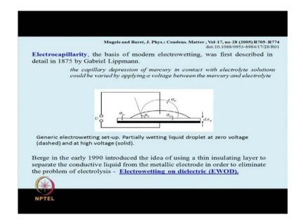
Now, this is classicalsetup figure of a setup wherein 1875Lippmann hasshown that there is sufficient or considerable depression of mercury whenit in contact with an electrolyte solution, and you can you can vary that depression of mercury meniscus by applying a voltage between the mercury and the electrolyte. But, as I said it is limited by the application of a very small amount of very small quantity of voltages.
