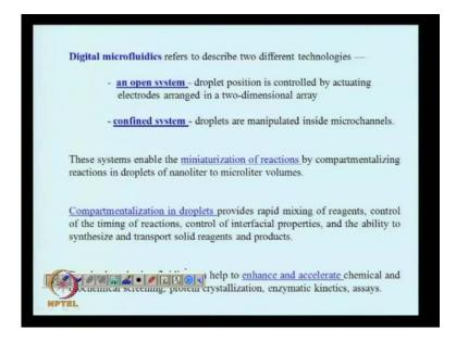
Now, a digital micro fluidics system can be can be of two different can be a fundamentally two different technologies. One is an open system and the other is in confined system.
