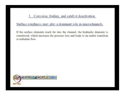
Now, the third point that I would like to discuss about it is pretty obvious straight forward is that surface roughness can play a very dominant role in micro channels. Any idea how much would be the surface roughness of a normal pipe orders angstrom millimeter microns? Just a pipe, which is carrying household water drinking water.
