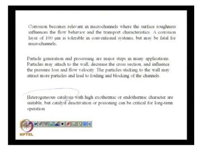
And corrosion also plays well fundamentally it basically, kills the flow through the micro channel. And there are several applications where you would see that the number of times a micro channel can be used is also limited. So, you do not you cannot use a micro channel for a reaction in which you have formation of particles may be nano particles and keep on using it without cleaning, because cleaning of a micro channel is extremely almost impossible.
