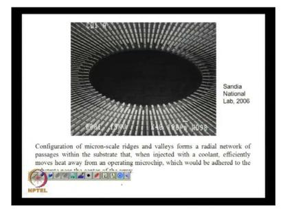
Which I have added to my last class is that this is a grooved a circularly, grooved wafer made in 2006 at this Sandia national laboratory. And what you can see there are channels, which will make the liquid flow from the outside from the periphery towards the center. And even in the next which you would see these, channels are not just unique single channels, in this channels there are other several channels which are also present.
