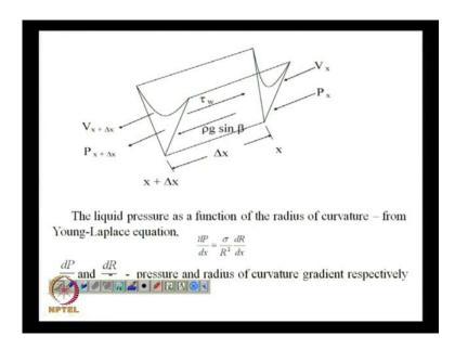
In the radius of curvature so, as long as we have a gradient in non zero gradient in the radius of curvature there will be some pressure gradient, which will cause the liquid to flow.
