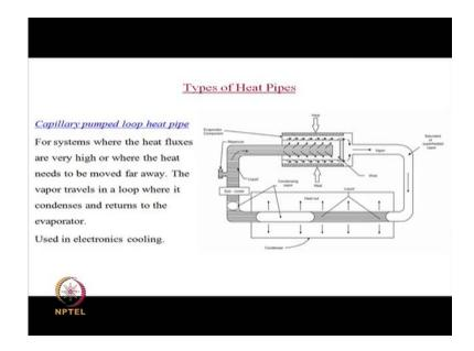
If we have very high heat requirement, that removal rate is very high, then there would be a capillary pumped heat pipe and these applications you can read in, read in a, any, any book on heat pipes and you would see, that these type of capillary heat pumps are also in use.
