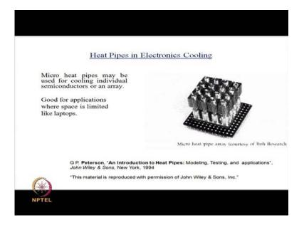
This is an array of heat pipe, which has been made for electronics applications and these are arrays of heat pipe where one side is going to be cold, the other side is going to be hot.
