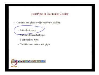
So, these are the 4 types of heat pipes, which are in use for electronics cooling, but in this course I am going to concentrate on the micro heat pipe only.
