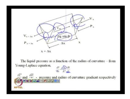
This is a very simple model of fluid flow in a, in a V-shaped micro channel and those of you who have done, all of you have done transport phenomena, just a simple shell momentum balance type of approach can be used to model the flow of liquid through a micro chip, through a micro channel in between two points where there is substantial difference in curvature.
