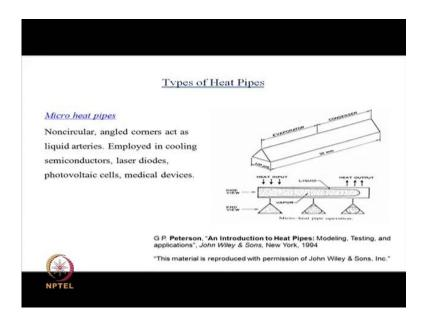
And suppose, you have transistor, a series of power transistors, which are bulky in size where you can still use wicks, you, you can keep them at the top and the heat is going to be let out from the bottom. So, the vapor from the top, vapor will flow from the top to the bottom and through the wicking action liquid will move in the reverse direction. So, against gravity it will go up, come in contact with the hotspot, evaporate and the vapor
