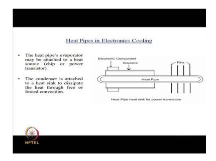
So, this, this is another example of heat pipe where this is going to be the cold, this is going to be the hot side and the heat pipe is embedded deep into it, and there are fins attached to the, to the cold side. And through convective cooling the temperature, or the heat temperature can be controlled.
