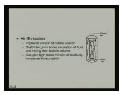
So, these are the different concept of air lift fermenter. So, it is improved version of bubble column reactor. Draft tube gives better circulation of fluid and mixing, than the bubble column. It can give high mass transfer and relatively low power consumption, what we have already discussed in this particular reactor system.
