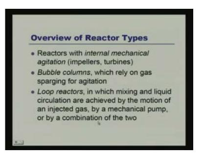
So, when we are going for that type of reactor selection, then, reactor with internal mechanical agitations, that is, impeller or turbine type of things are there; sometimes bubble columns, that is, which rely on the gas to sparge for agitation and sometimes, we are looking for the loop reactor, where we can tell that, this here, this mixing of the liquid circulation are achieved by the motion of an injected gas, by a mechanical pump, or by a combination of the two.
