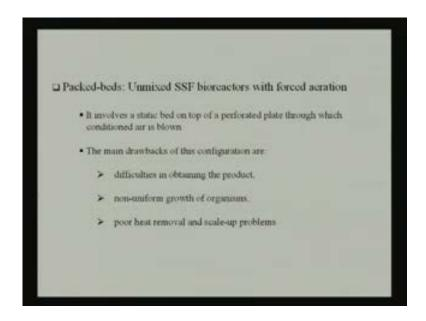
Now, when we are talking about the packed-bed unmixed solid state fermentations bioreactor, it involves the static bed on top of the perforated plate, through which the conditions air is blown. The main drawback of this configuration is that, it is difficult in obtaining the product; that means, leaching out the product is difficult; non-uniform growth of the microorganism is also there; poor heat removal and scaling up problem are associated with this.
