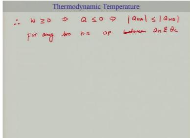
So, that leads to the statement or this means that W has to be greater than equal to 0, which means that Q has to be less than equal to 0 and this implies your Q H A should be less than equal to Q H B. This is for any two heat engines operating between theta H and theta C. So, this is what we can come up with this exercise.
