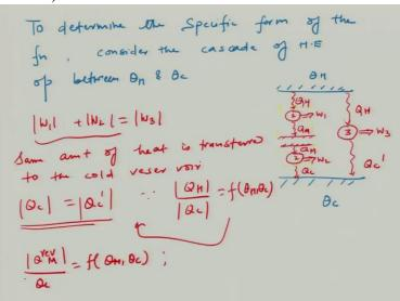
So how do you determine the function? So, to determine this function f here, specific form of the function, what we are going to do is we are going to consider a cascade, consider the cascade of the heat engine okay which operates between theta H and theta C. So, the way we can do that is the following. We can just consider this theta H, this is the thermometric temperature and this is your again theta C and now we can consider heat engine 1, this is 2 and this is your 3.
