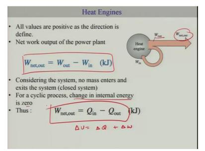
So this is what we are saying this is a net work. So, heat engine is a cycle here and effectively W out some part of W out can be considered as the part of the W in which is used by the pump.
