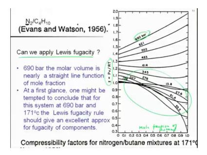
So, this is an example taken from the literature due to Evans and Watson and the data is 1956 data. So, what we have is the following that this is compressibility factor right as a function of the composition of nitrogen and beauty the nitrogen is close to 0.9. So, this is a basically the compressibility factor as a function of mole fraction of butane ok. So, this is the data directly from Evans and Watson work in 1956. So, the question is can we apply Lewis fugacity rule here.
