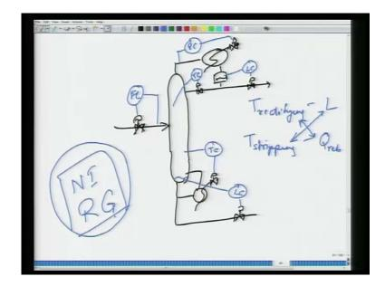
For example, if you take a distillation column here is the distillation column, a simple distillation column and do not worry, if you do not understand some of the things, that just an example. Reflex drum you put in some reflux back into the column, take out some distillate, where some reboil you are putting in steam here, that cause the vapor to boil up, and then you are taking out the bottoms.
