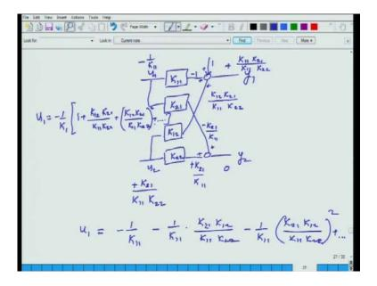
So, that steady state change is essentially the gain given by the gain. Let us say I have got K 1 1, K 2 1, K 1 2. So, let us say I am paring 1 with 1, 2 with 2. So, 1 is paired with 1, this goes like this, and this goes like this. What I am doing is, I am paring y 1 with u 1, and I am paring y 2 with u 2. And let us say I do not have a control system; but let us say I am an operator. If I am an operator, and I am told; look boss you have to maintain y 1 and y 2 had set points.
