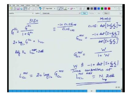
Now, let us talk about multivariable tuning. How do we do SISO tuning? What is the basis of SISO tuning? SISO tuning is what? You take G open loop divided by 1 plus G open loop. Define this as G closed loop. And then what you do is, 20 log on base 10 of G closed loop. you define this as L C L or L close loop and then what you basically do is, adjust K c such that L C L max is equal to 2 d B. That is what we do right?
