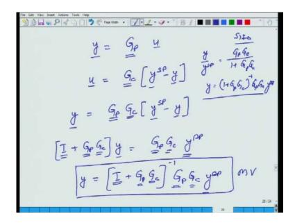
So, what I had was y is equal to G p matrix times u, and what I had was, u is equal to G c matrix times y set point minus y vectors. When I substitute for u, what I will get is, y is equal to G p G c, and please note here that the order of matrix multiplication is important
