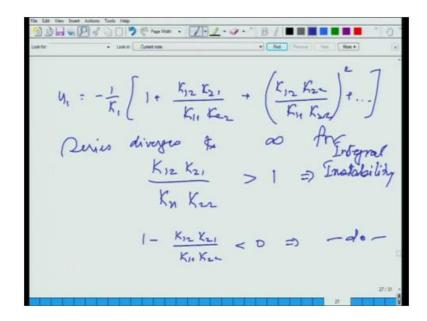
u 1 has to change by this guy. 1 plus K 1 2 K 2 1 divided by K 1 1 K 2 2 plus and K 1 2 K 2 2 divided by K 1 1 K 2 2 whole square plus and so on, so forth and infinite series. This infinite series will converge to a finite value if and only if, K 1 2 K 2 1 series converges, for converges to a finite value. Converges to a finite value, for this multiplication factor being less than 1.
