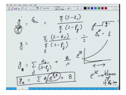
If I look at the closed loop transfer function or if I look at any transfer function if I look at any transfer function closed loop open loop whatever. So, for example, y over y set point any transfer function then it will be a bunch of poles and zeros. So, so let us say this is product of some bunch of zeros and a product of some bunch of the denominator
