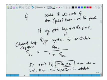
So, what this basically gives is that stability of a system if you have a system and weather transfer function G this transfer function is stable if all roots of denominator which are also referred to as poles have negative real parts what this means another way of looking an at looking at it is if any pole has.
