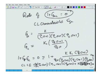
So, if you want to figure out whether a closed loop system is stable or not then what you need to do is figure out roots of 1 plus G open loop equal to 0 stability is governed by the roots of this equation this is called the closed loop characteristic equation. So, now, what you want to do is figure out whether this guy has any root in the right half plane if it has any root in the right half plane the closed loop system is gonna be unstable.
