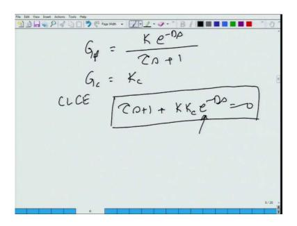
So, a very typical transfer function would be G p is equal to first order plus dead time K times e to the power minus dead time upon tau s plus one now if you look at this guy the closed loop characteristic equation for a p controller. So, and let us say G c is equal to K c; that means, it is a p controller if it is a p.
