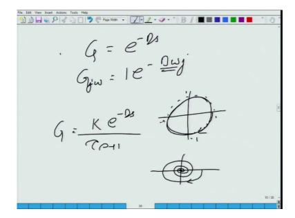
So, G is equal to e to the power minus D s and G j omega replacing s by j omega will be e to the power minus D omega j right what is the magnitude of this guy well the magnitude of this guy is one all the time what is the angle well the angle is minus D omega and as omega increases the angle becomes more and more negative what you get is magnitude is one.
