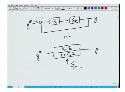
So, what we have is the simple feedback control system G c G p this thing can actually is actually equivalent to this is the y a single the above block diagram is equivalent to this simplifies to this and this I will call the closed loop transfer function.
