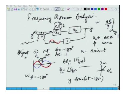
It is and the amplitude ratio is given by AR is equal to at some frequency omega is magnitude of G j omega that relates the transfer function and phi is equal to angle of G j omega at that frequency this is what I told you, but please note since the feedback loop is not closed G in this case is nothing, but G c G p G c G p and I am looking things out here. So, I am looking at this guy and. So, what was I trying to say I was trying to say you are plotting G j omega as a function of omega.
