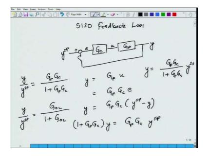
So, let us look at SISO systems; a SISO single input single output feedback loop. If you look at the single input single output feedback loop; so you got your process it has a transfer function G p, you have a controller, which has a transfer function G c, and you got the output the output is compared with its set point negative feedback, and that is it; that is your single input single output control loop. And this is called the error this is the control input and of course, that is the output.
