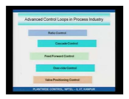
Last time we were looking at advanced control loops that are very commonly used in the process industry namely ratio controllers, cascade controllers, feed forward controllers, over ride controllers, continue and discuss over ride control and valve positioning control, over ride control. Well over ride control like the word indicates an overriding circumstance occurs during process operation which can potentially result in a safety hazard.
