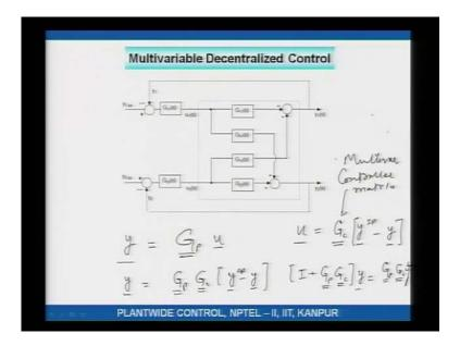
Now, so this is my multi variable 2 by 2 process and what I am now doing is controlling output 1 using input 1 and controlling output 2 using input 2. What we then have is this is actually called a decentralized control system and to understand this a little better, let me just say that what we have is y is equal to G p matrix times u. u being the input vector input. This input is error times a controller. So, u is equal to a control matrix time's error.
