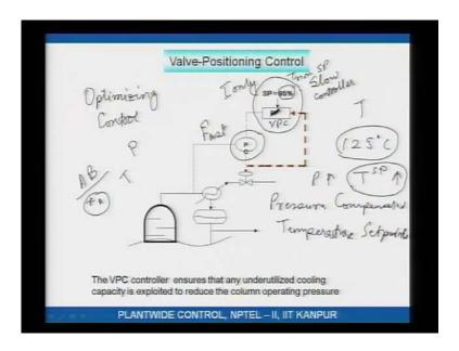
Optimizing control, that is by implementing valve positioning controllers what you are trying to do is either minimize steam consumption, minimize electricity consumption. Another place that I know it is used is to maximize production or you know maximized throughput optimizing controllers are also used in that application we will talk about that through the course, but the point is valve positioning control is routinely employed in order to make your operation as economical as possible.
