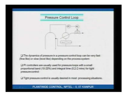
Pressure control loops, well dynamics of pressure loops can be as fast as slow loops for example, if your are for example, gas coming out of a cylinder or for example, gas coming out of a vessel you change the valve position, and the pressure responds immediately right. So, the dynamics of the pressure, open loop dynamics of pressure can be very fast; that means, the dynamics is flow like or it can be very slow; that means, the dynamic is level like depending on the process system.
