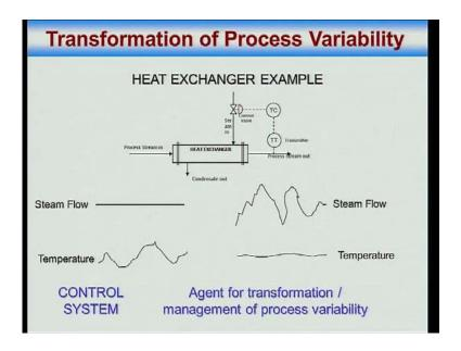
How do we structure? Now, that is the next thing that, that I am going to trying to explain here, it is a heat exchanger, it is a heat exchanger. You got a process steam going in, and process steam going out, steam is being use to heat that heat exchange, that process steam.
