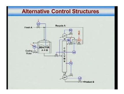
Now, I want to show you that, there are different possible control structures even for the simple plant, what do you, what do you have here an isomerization reactor A goes to B, exothermic reaction heat is being removed by cooling water, B is heavier than A. So, the column recycles A at the up the top, and B is taken down the bottom, and the stripping section essentially make sure that a does not contaminate B, this is your process.
