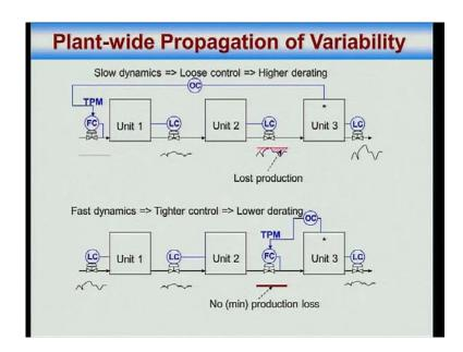
Now, let us see how do we structure control system? So, here is the 3 unit in series process we have seen, this before in number of times I set the throughput here, level control then has to be in this way in the direction of process flow, unit three is start, so it is the bottle neck unit; that means, that means this unit cannot handle more than a certain amount of flow, there is capacity constrain on unit 3.
