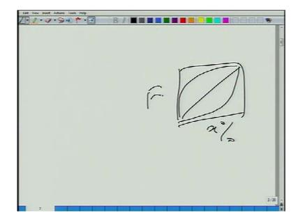
So, x percent versus flow rate right, valves are non-linear, because valves are non-linear, so flow control will be always fast, you changed the valve position flow will immediately response, so you can tune the controller to give you whatever flow you want and within half a minute, it will give you flow that you want kind or like if you are opening a tap in half minute, you will get flow that you want exactly right.
