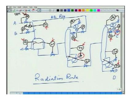
So, last time what we saw was, we were trying to draw controlled structures for the simple process, one reactor two column process. And we drew a non-demand controlled structure; we drew a controlled structure with the reboiler duty in the recycle column, which is the first column as the throughput manipulator. Now, today let us draw a conventional minded control structure for this process, what do I mean by conventional minded, what I mean by conventional minded is...
