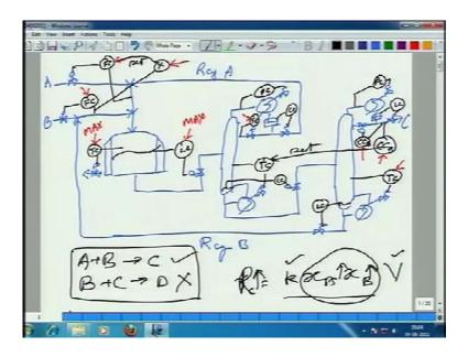
So, welcome to this next class. I think last time, we will looking at the same thing A plus B goes to C is just that, C is intermediate boiling and so you had to have two destination columns right, to do the separation. And we do the light out first (()), which means the lightest component is separated out first; why did we do that well may be a doc cycle something, so you want to remove it first so that. So, this is A recycle.
