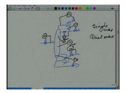
So, we are looking at column, and I was think of simple drawing a control system for it. So, this is my column distillate, this is my re boiler and we got the bottoms, heat is given you got the reflux, well may we do this latter on, you got the steam, and now let us put it in this the control system for this guy.
