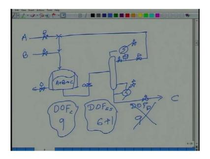
But let us now, so here is the process A plus B goes to C no side reaction it is a hypothetical process or let say negligible side reaction, the reactor the fluent contains A B and C, C is the heaver component, so it is goes down the bottoms of the column.
