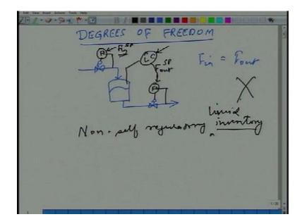
If I look at the steady state material balance around this tank, I know that flow in must be equal to flow out. What that means is, of these two independent valves, of these two independent flows, there is you know two independent valves only one can be set, only one flow can be set independently. The other flow for steady operation must equal you know you know you know whatever flow you have set, so only one of these flows can be set, the other one must match whatever has been set yes or no.
