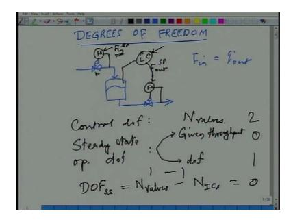
So now, we come to, what is called controlled degrees of freedom, what is controlled degrees of freedom? Controlled degrees of freedom is number of valves, number of independent valves. How many valves are there in the process, that can be adjusted then there is so what is the controlled degrees of freedom for this process, 2 for this simple example, it is 2.
