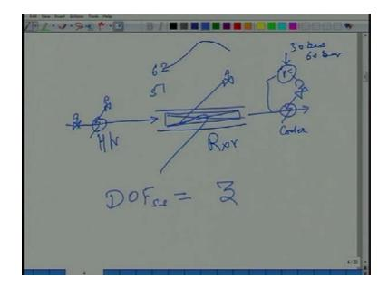
So, this is the reactor, this is the heater, that is the cooler so you can set the flow through this train only at one place. Because it is essentially a pipe and there are no drums or surge drums or you know large hold up's anywhere, is essentially flow through pipe. So, you cannot put a valve here similarly, you cannot put a valve here, either etcetera, etcetera. So, feed valve is discounted because through put is given, total number of valves is then 1, 2, 3.
