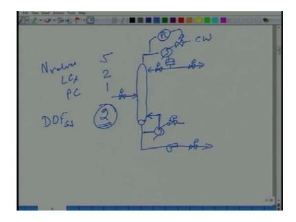
So, here is a simple distillation column, I have got a feed of course, it has a valve however, I am not going to count it because this feed is being set by an upstream process, it is not in my hands. Vapour, condenser, reflex drum, reflex distillates, there is liquid that accumulates at the bottom, I have put in some steam sorry before, I start asking you questions, I want you to know that, this is the distillation column right.
