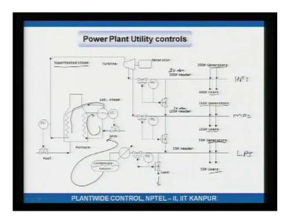
Power plant utility controls well. Why is this called power plant? Yes, because you are having that generator there. This is the steam unit in in in a large petrochemical complex. What you have is you have got a furnace and you are let us say burning diesel or fuel gas in that furnace. Water goes into the hot tubes which are exposed to the fire in the furnace of course, sorry it is it is going like this. So, the liquid water heats up, comes
