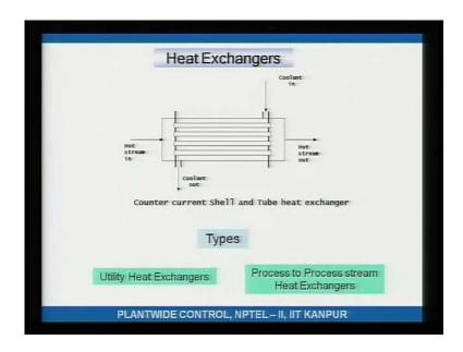
So for example, what you have here what is shown here is, there is a hot stream coming in goes into the tubes and comes out the tubes. Then you got coolant going in counter direction. So, the hot stream gets colder and the cold and the coolant gets hotter. There are two types of heat exchangers, utility heat exchangers and process to process stream heat exchangers, and we will just see what they are as we go along.
