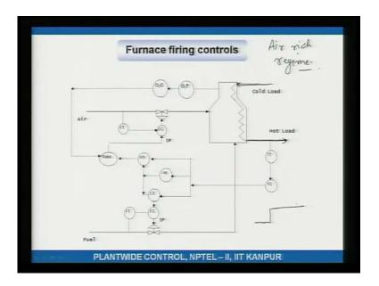
The first one will do is furnace firing controls, see here is a furnace. So, you are putting in air and fuel the fuel burns in the presence of air therefore, the tubes are really really hot. The cold process stream that is flowing through the tubes gains you know you know through those hot tubes becomes hotter and flows out. So, this is cold in this is hot out. So, this is the process stream that is being heated process stream comes in cold stream
