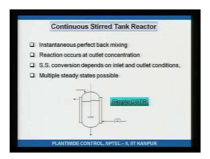
Well in a continuously stirred tank reactor well there is perfect back mixing, what that means is that the exit concentration is the same as the inlet concentration and the concentration inside the reactor concentration temperature, and all other state variables if any are the same at every location in inside the reactor.
