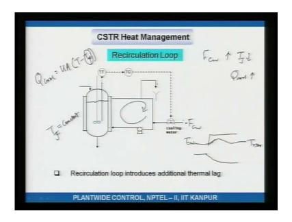
On the other hand if you did the same thing, if the same thing happened here you know T cooling water goes up as a step, well then what happens? Cooling water is hotter therefore, the jacket is hotter because the jacket is hotter less less than necessary heat gets removed across the walls of the reactor therefore, reactor temperature starts to rise. As the reactor temperature rises in response to the feedback action of this temperature
