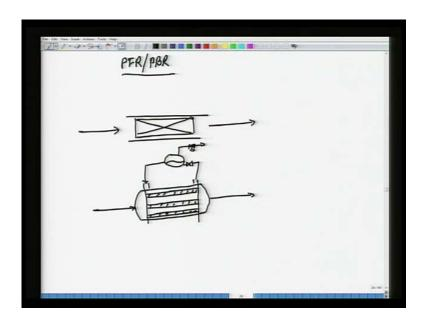
We have been looking at plug flow reactors or packed bed reactors and what we saw last time was adiabatic operation. So, here is a catalyst loaded tube, heated feed comes in, heated feed goes out, reaction occurs in this bed, then we also saw that adiabatic operation especially for highly exothermic reactions will cause the temperature to rise too much and that would not be good for the health of the catalyst. Therefore, one of the most common configurations is a shell in tube heat exchanger.
