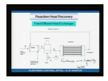
When I put in the temperature controller what happens is if this temperature goes up sure this temperature goes up, but then this temperature goes up therefore, this goes back down and therefore, this temperature goes back to its you see what what that does is the temperature controller essentially stabilizes my system. So, this is an example of a control system stabilizing an open loop unstable system.
