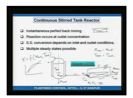
Now, we get to the other type of idealized reactors that are that are very commonly, that almost all chemical engineer should be familiar with all chemical engineer should be familiar with, it is called the continues stirred tank reactor. Well, I have I have noted a few points here there, there are actually pretty straight forward. This stirrer is essentially
