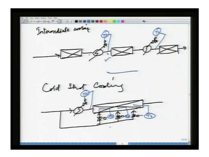
So, here is an adiabatic bed. You are, you putting in reactor feed because the reaction is exothermic, but not highly highly exothermic. Therefore, temperature rises, you cool it off, send it again, temperature rises, cool it off again, send it to the next packed bed. Sometimes, this cooling is also necessary to see in equilibrium reactions if you cool the
