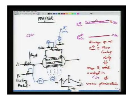
On the other hand if you got a temperature profile, let us say which looks this is length of the reactor, it is temperature if the hot spot occurs early. In this case if the hot spot temperature is increasing will this temperature increase or decrease? Well, you really cannot say. Even if the hot spot temperature is increasing it may be that the that the exit temperature is decreasing. So, you cannot really say what will happen to the exit temperature.
