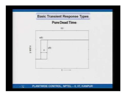
Basic transient response types pure dead time, so you make change know that happens of the output after some time output goes to same value as the input, so there is of pure dead time and this is because of transformation lags.
