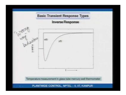
Here is an inverse response, u give the step change, the output goes in the wrong direction first, in the other direction first, turns the round on and then goes back up, so the initial direction of response is in some sense, the wrong direction; this is also some time refer to us wrong way the behavior, wrong way behavior; another common example of inverse response of chemical process is is the level inside boiler in example of inverse response process.
