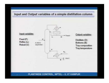
So, hear is for example, distillation column if there is a feed to the column, let us say it is an A B C mixtures, A being the lightest component, B being intermediate boiling, and C being the heavy component and you are doing a direct split, so what; that means, is you
