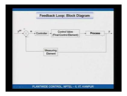
You have the process, there is sensor that is measuring the output, this is a measuring element through the this includes transducer, this is saying what the output is, what may
