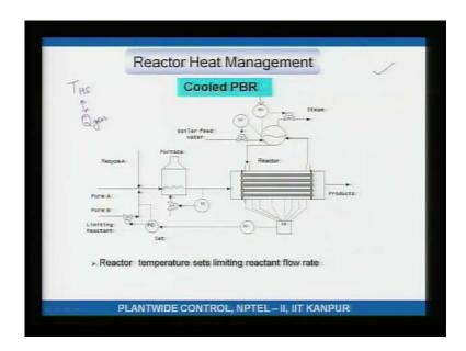
After this I will end alright. In this third scheme everything is the same except that the temperature controller instead of adjusting either the pressure set point or the reactor temperature in is adjusting the limiting reactant flow rate. How does this work? Well this works as follows if the hotspot temperature is increasing, that means you are generating
