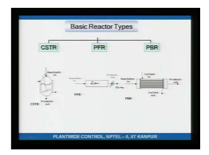
You will know that reactors are actually categorized into three basic types; the CSTR which is the continuously stirred tank reactor, the PFR which is the plug flow reactor, another variant of the PFR is the PBR which is called the packed bed reactor. The difference between PFR and PBR is plug flow reactor is like a hollow tube - a hot hollow
