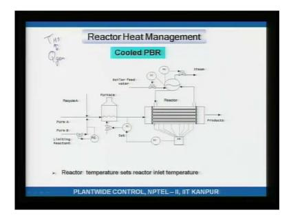
You see. So, in this case works by Q gen so, T hotspot is controlled by adjusting the amount of heat that is getting generated due to reaction Q cool is not getting manipulated I hope this difference is clear. There is a third scheme and here is the third scheme.
