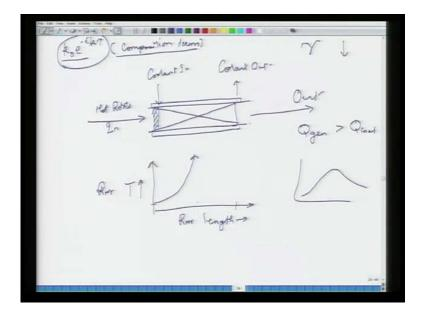
This is where you know the flame is burning in a controlled fashion. So, to speak so, these are the three different states which a packed bed reactor or a plug flow reactor can have.
