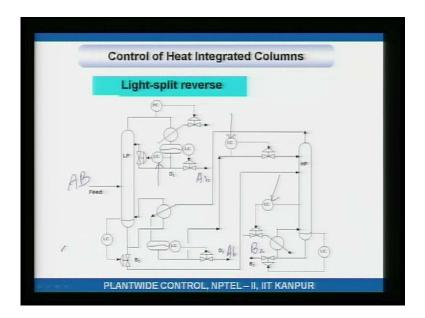
Over here, and again notice that again notice that there are three compositions, that are being set 1, 2, 3 and I check, well if this is another A B mixture like I describe to earlier this is A with a little bit of b, A again with the little bit of b, and this is B with the little bit of a, why was the degrees of freedom 3 here and 4 in the previous case.
