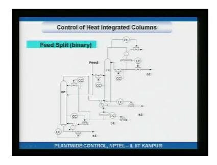
So, here is the feeds splits binary distillation column, that I just explained to you, and you would have appreciate is the same thing is the D 1, 2, 3 and is the fourth one, where is the fourth one there is a fourth one, these 4 set points is what the operator adjust to get the kind of split, that you want.
