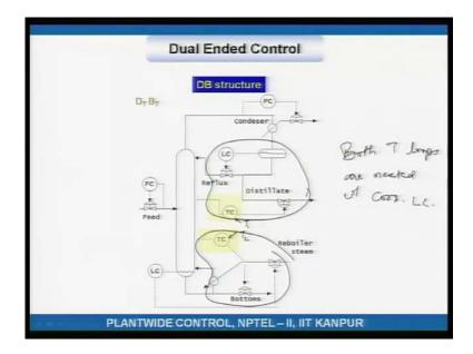
Yeah again here T 1 T 2, notice both loops are nested, both T loops temperature loops are nested with corresponding level controller.
