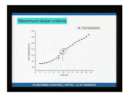
So, this is the maximum slope criteria if I look at it I may want to control this tray temperature because this is where of course, the feed is here, you never control the feed tray because temperature of the feed tray may change because of two reasons either the condition of the feed is changing that means the feed is hotter or colder, that would cause a change in the temperature on the feed tray or the separation itself is changing.
