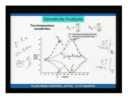
If the sensitivity plot looks like this I would not go for dual ended temperature control. So, on such a column where the sensitivity plot is like this I would recommend single single ended, single ended. If my sensitivity plot is like what it is shown here, well this sensitivity analysis is showing that there are indeed two locations that are highly sensitive and therefore, they should be reasonably independent and I may control this tray temperature and this tray temperature.
