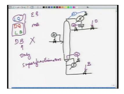
And in that case in that case the level controller at the top has to be oriented this way, level controller in the bottoms has to be oriented this way, and then the operator sets the distillate and the bottoms and this is called the D B structure, it is never used in practice, it is seldom, it is used only in super fractionators and never elsewhere, and that is because this structure valve its material balance in the sense that distillate plus bottoms must always be equal to the feed.
