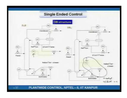
Here it is, is another example of a nested loop, nested with bottoms level controller. Maybe I can get another one L B structure, this is again nested, is that an example of a nested loop here let us see.
