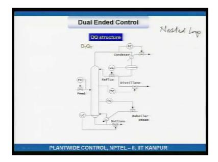
If you are trying to do dual ended control on a material balance structures that means D Q or L B or even D B that means you are trying to control two tray temperatures in these basic control structures there would be a nested loop and what do I mean by a nested loop?
