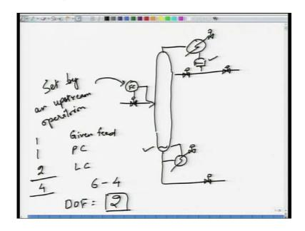
Good morning and welcome to the next lecture. We have been looking at distillation columns and just to recap what we have done, if you look at simple distillation column where the single feed and two product streams. What we saw last time was that there are a total of 1, 2, 3, 4, 5, 6 valves, independent valves on the column, and the feed is typically set from upstream set by an upstream process, an upstream operation typically a reactor.
