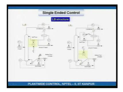
Keep on going the same way, this tray temperature is being set by the operator in order to maintain this tray temperature the reflux is being adjusted and of course, the bottom steam flow rate is being set by the operator. The other variant reflux is being set by the operator and a tray temperature is controlled by adjusting the bottom stream.
