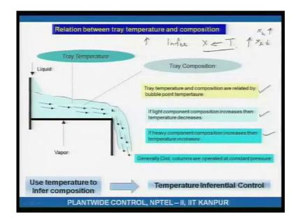
Most columns you infer composition from X from the temperature and and what is the idea behind this, if on a tray the composition of the heavy component is increasing what do we expect would happen to the boiling temperature of that liquid in which heavy is becoming more and more, you would expect that boiling temperature of that liquid will go up. Similarly, if on that tray the composition of the light component is increasing its boiling temperature will go down.
