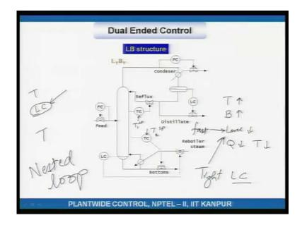
Let us look at the nested structures here. Operator sets this set point layer T 2 by convention. Let us say T 2 is increasing, what that means is heavy material is accumulating inside the column. What I would do then I would like that heavy material
