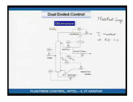
T 1 T 2, so, T 1 is nested with reflux drum level controller. If I call this T 1, if I call this T 2.
