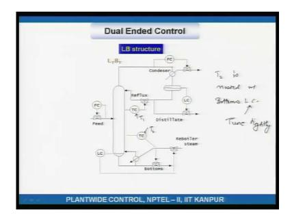
T 2 is nested with bottoms level control. Therefore, this should be tuned tightly, you can also have a nested loop in a in a single ended controlled structure. Let me go back and see if we can, yeah.
