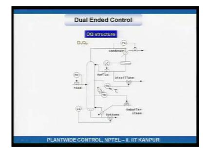
This is the dual ended temperature control variant of the D Q structure. Well, operator is setting this and this. However, the manipulation handle that is used in this case is distillate rate. In this case it is it is the re-boiler duty. T 2 is controlled as before using the boiler duty.
