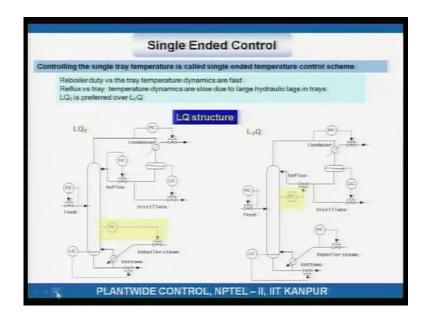
So, it is written here re-boiler duty versus tray temperature dynamics are fast, reflux versus tray temperature dynamics are slow, therefore L Q T is preferred over L T Q that is usually the norm.
