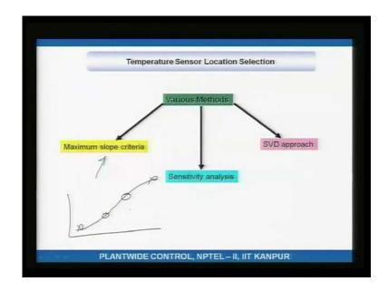
I just discussed with you the maximum slope criteria, what we are trying to do here is look at the profile wherever the slope is maximum or large at least the slope should be large that is a decent location for the tray temperature to be controlled. So, you would like to control a tray temperature for example, here may be here, but certainly not here, certainly not here.
