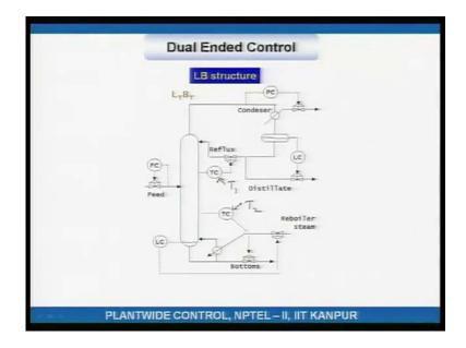
Here what we have is again two tray temperatures are being set T 1, T 2. T 1 is controlled in the usual way using reflux, T 2 is controlled using bottoms and that is
