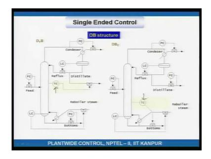
We keep going ahead D B structure well either you can control a tray temperature by adjusting the distillate or you can control a tray temperature by adjusting the bottoms.
