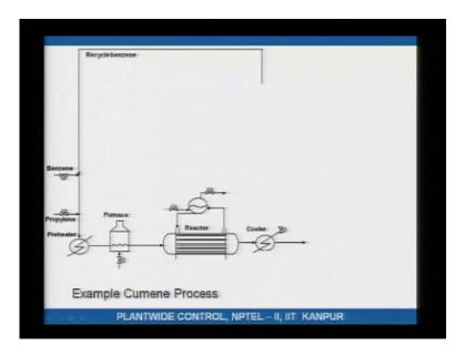
So, this is the reactor, the reactor affluent is cooled, the un condensable do not condense, the benzene, the diisopropyl benzene and the cumene they actually liquefy.
