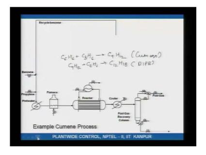
Just to give you an example of chemical processes is, here is an example process for cumene manufacturing, it is slightly simplified. So, what you have is what you have is propylene and benzene being pre heated, vaporized and then heated to the reaction temperature, which would be say around 350 degree Celsius in a furnace. The benzene is also being mixed with un reacted benzene which comes, which is being recycled.
