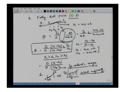
So, falling rate period, now we are talking of C to E, all right. All the way till its falling of course, they are two regions. 'a' where the curve is linear starting from critical moisture content, its c to this d, which is x d.
