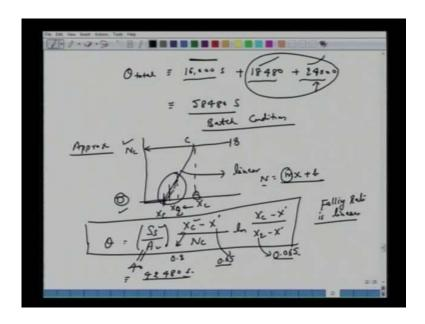
So, we have three, all three times, total time for drying. First, we had number for constant falling, constant rate which was 16000 seconds. So, this is the rate at, this is the time over which the rate which remains constant moisture dries at a constant rate.
