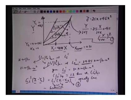
We have capital X and capital Y. So, that is where we have been working, trying to plot, do the calculation based on solute free basis. So, if we have equilibrium curve given as small y equals 2.5 x plus 4.5 x square, we can write it as y over 1 plus y equals 2.5 capital X over 1 plus x plus 4.5 x over 1 plus x square.
