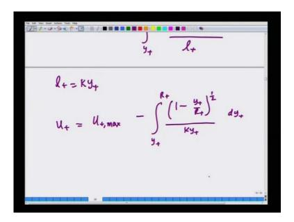
Now, l plus is k y plus this is the prankdial's hypothesis for the mixing length being a function of the distance from the wall. So, u plus is nothing but, u plus maximum minus integral y plus R plus times 1 minus y plus by R plus to the power half by k y plus d y plus. So, all we are saying is that when l plus is large compared to 1, we are expanding this term and that is the only simplification that we are making, when we do this whole exercise that is the only simplification we are making.
