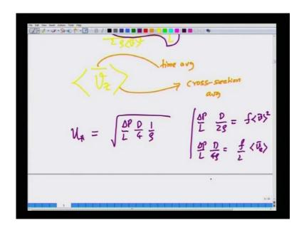
So, I will get u star the scale used for non-dimensionalization is nothing but, square root of delta p by L d by 4 1 over rho but, delta p by L times d by 2 rho is f times v square. So, delta p by L d by 4 rho is nothing but, f by 2 v z so, v z square.
