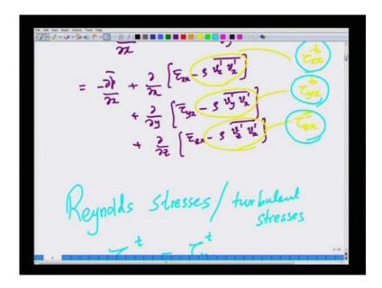
Now, these three so, can be again included back into this derivative minus partial p bar by partial x plus partial by partial x of tau x x bar minus rho v x prime v x prime plus partial by partial y tau y x bar minus rho v y prime v x prime plus partial by partial z tau z x bar minus rho v z prime v x prime put 1.
