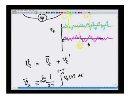
And if we you measure for example, the z velocity as a function of time using some probe at a given point in space in the pipe, you will find that there will be a large amount of fluctuations about the mean.
