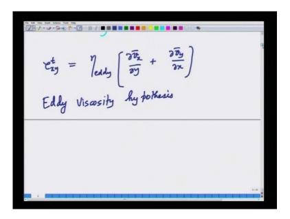
So, one option is to write turbulent stress in terms of a viscosity called eddy viscosity. Times the mean velocity gradients just as we wrote for the viscous stress this is called the eddy viscosity hypothesis, this is not a rigorous relation, this is merely hypothesis. So, this is called a eddy viscosity hypothesis.
