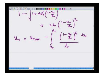
Now, so we can further. Therefore, write u plus as u plus max minus integral y plus to R plus 1 minus y plus by R plus to the power half d y plus divided by 1 plus.
