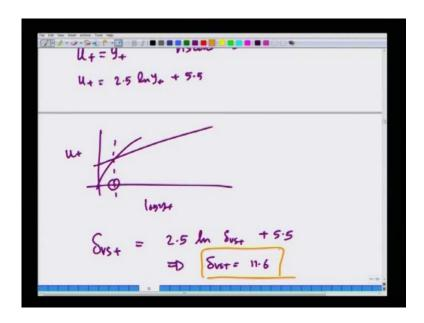
Now, if you plot these two curves and then say that the region where these two curves meet is the thickness of the viscous sub layer. Then so, you will have u plus as a function of log y plus, we have one (()) total like this, another (()) total like this.
