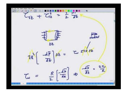
So, tau r z bar plus tau r z turbulent is d p d z R by 2 plus c 1 by r now, we can readily say that as r goes to 0 in the center of the pipe the stresses will be finite so c 1 has to go to 0. So, we can say very easily that tau r z plus tau r z turbulent is R by 2 d p d z. Now,
