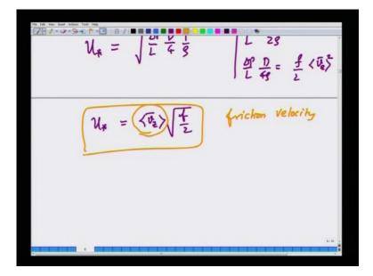
So, if you substitute this in here you will get u star is v z average square root of f by 2. So, this is a highly non-trivial velocity scale this is called the friction velocity because, normally we would non-dimensionalize things only by this. Here we are trying to multiplied by square root of f over 2. So, it is highly non-trivial in terms of nondimensional using turbulent flow.
