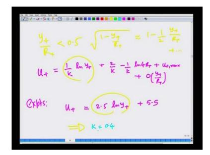
Suppose, you have y plus by R plus less than 0.5 you can expand the square roots, so root of 1 minus y plus by R plus is approximately 1 minus half y plus by R plus, plus so on.
