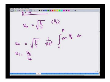
Now, we have all the required quantities to find the friction factor versus Reynolds's number relation. Now, you know that u star is square root of f by 2 v z, so this is nothing but, square root of f by 2 the definition of v z is 1 over pi R square 0 to R 2 pi r the time average velocity v z bar d r. And this is u star we know that u plus is v z by u star this implies.
