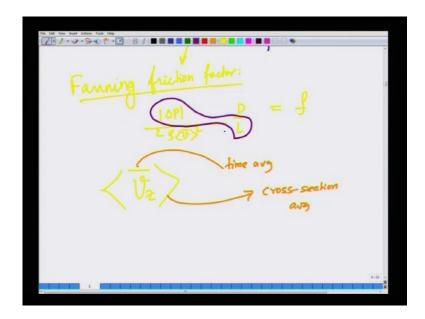
So, here I am going to use the Fanning friction factor which is differs by a factor of 4 from the Darcy friction factor which we have already pointed out the differences Fanning friction factor is defined as delta p divided by 2 rho v square times d by L is equal to f this is the Fanning friction factor. Now, there are 2 types of averages that are involved suppose I have a quantity, v z the over bar denotes a time average, the angular brackets denotes cross sectional average.
