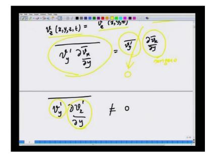
But, we will also encounter quantity such as this, the product of two fluctuations average and this is not 0, the product of two fluctuations is the average of two product of two fluctuations is not equal to the product of their averages. And this is because of the factor these two quantities could be correlated in time. So, when you integrate over particular instant particular extent of time they could in general be non 0.
