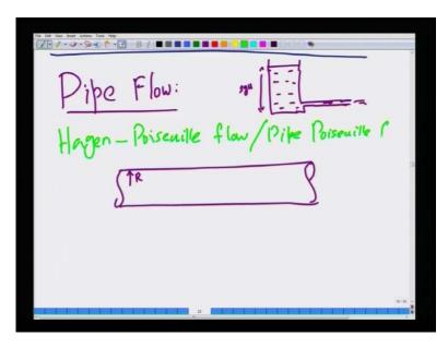
So, imagine having a long pipe, a rigid pipe, a circular pipe or radius r radius of the pipe is R, and this ends of the two pipes are let us, you have one end of a pipe is connected to a huge reservoir, and the other part end of the pipe could be open to a atmosphere. So, because of this virtue of this pressure head present in this. Let us say liquid is present fluid is present here, and because of by the virtue of this gravitational pressure head rho g H.
