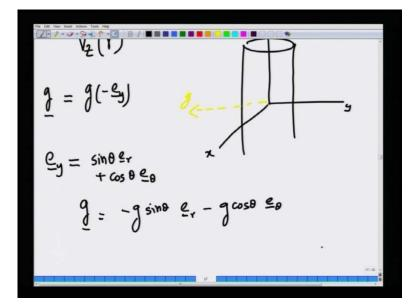
So, what we have ended up this with the fact; that you have a velocity field steady, velocity field v z, it is a function only of r direction. It is not a function of theta direction axis symmetry; it is not a function of z direction, because of fully developed flow
