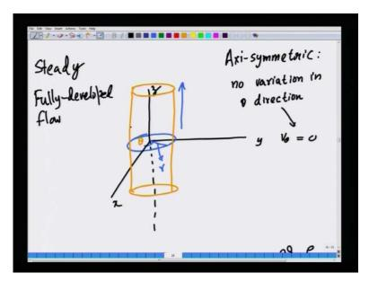
Let us, first draw the coordinate system; this is x y and z, if you have a pipe, you can nicely place the center of the pipe; you can align the center of the pipe with the z axis, with the z axis. So, you can nicely align the center of the axis of the pipe with the z axis. So, you are exploiting the symmetry of the pipe by just nicely placing the axis of the pipe along with the z axis of the cylindrical coordinate system.
