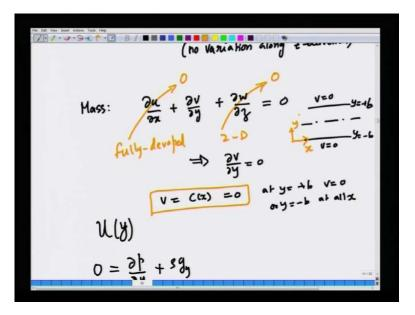
So, there is only one velocity U in the flow direction, and it can be a function only of the normal coordinate y. So, this is the information; we have so, far obtained from the continuity equation. Now, we will go to the x momentum equation, the y momentum equation, will simply tell you that partial p partial y plus rho g y is 0. If you align the gravity vector in this fashion; let us, this say is x, this is y, if gravity is acting in this minus y direction, then g y is minus g.
