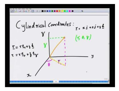
So, we quickly explain, what is the cylindrical coordinate system, you have a 3 cartesian coordinate vectors x, y, and z, any point in space is from the origin; you connected how is it described in cartesian coordinates, we decompose it into so, let us try in cartesian coordinates any position vector is x i times i plus y times j plus z times k.
