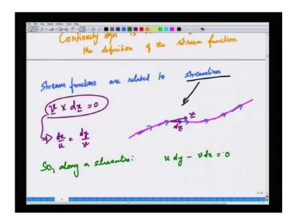
So in that sense, a stream function is very very helpful in the solution of two dimensional incompressible flow problems. So, it is a purely mathematical reason has to why this I mean this motivation of stream function is purely mathematical. In that of course, it simplifies the solution of equations by reducing the number of equations by one.
