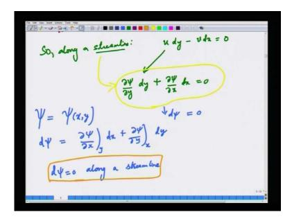
So along us stream line along the stream line, we can say that u dy minus v dx is zero. This is along the stream line from the definition of the stream line. Now, I am going to use the definition of the stream function that u is partial psi by partial y dy v is minus
