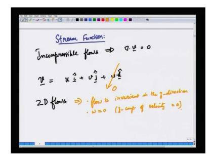
Now, we going to go further proceed further, and we are going to introduce a notion of a stream function. Now, I am going to assume again incompressible flows. For an incompressible flows, we always has del dot v is zero. In general, fluid flows the velocity vector, velocity is a vector can have component in the i direction plus component in the j direction plus a component in the k direction; that is the z direction.
