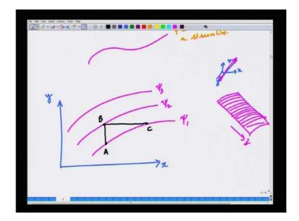
So you have a 2 D flow domain in the x y plain, what we mean by say, what we mean by two d flow is that the variation long suppose we have x, y and z. The variation along the third dimension z, this is the x is less very very less, so there is no variation in the third direction. So that is the meaning of saying that flow is two dimensional.
