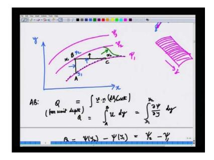
So, q is simply integral A to B u dy. and what is the differentiating thing between points A and B. it is the y coordinates, this is y 1, this is y 2. So this is simply y 1, simply equal to y 1 to y 2. Instead of u, I can put partial psi by partial y t y. so q is nothing but, psi at y 2 minus psi at y 1. So and psi at y 2 is simply psi 2 and psi at y 1 is psi 1, because along each and every point in this line the stream function is a constant psi 1.
