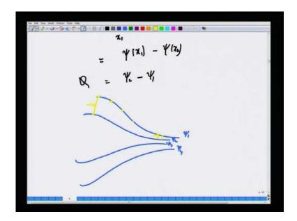
So if you take any two orientation, the amount of fluid that flows between these two points per unit width of the third direction per unit time is always given by the difference in the value of the stream functions between those two stream lines. So, this the difference in values of stream function between any two stream lines directly gives you a measure of how much volume of fluid that is going to flow between those two points between those two points.
