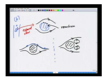
Another example is the case of a catalyst pallet which I just mentioned. Suppose you have a catalyst pallet inside a packed bed. So, let us look at a pack bed which has many pallets, but let us take one pallet and expand the view around a pallet. So, fluid is flowing like this, so fluid is flowing like this. So, the rate at which reactants are brought to the surface and let us say the reaction happens at the catalyst surface. The rate at which the
