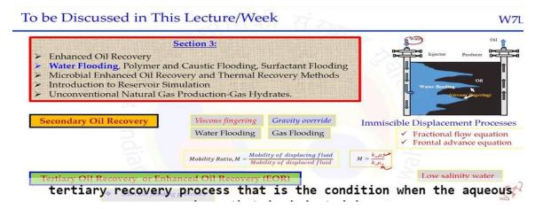
So the mobility ratio is the ratio of displacing fluid divided by the mobility of the displaced fluid. So, basically it is the ratio of the parameter where the mu o is in the numerator and mu w for the water injection in the denominator. So we can see the mobility ratio should be favorable when the m value is lesser than 1 and in certain cases
