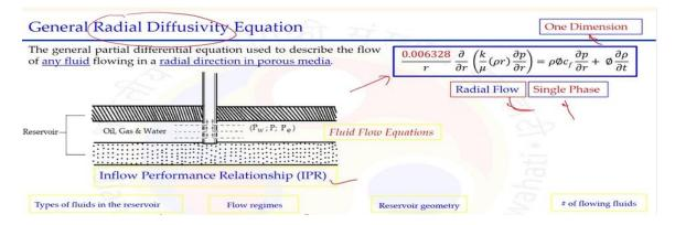
But for the simplicity purpose let us discuss the case of linear flow as an example. In linear flow what is happening fluid is flowing only in one direction we can take a control volume here in this control volume of the del x thickness the fluid is flowing from x to x
