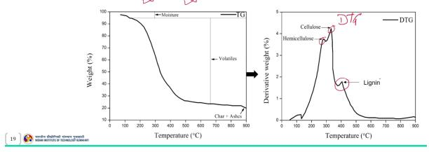
Similarly, the structural composition of the biomass can also be estimated using the thermogravimetric analysis method. So, as we discussed in the previous slide as well, the DTG plot helps to identify various conversion steps at different degradation rate here in the specific DTG plot.
