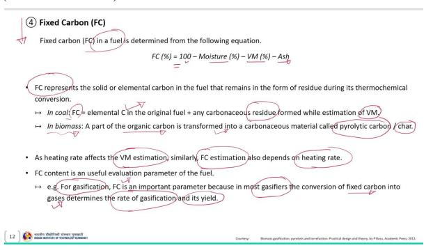
So, next in the approximate analysis list is the fixed carbon content. Fixed carbon in a fuel is determined from the following equation and it is 100 minus moisture percentage, volatile matter percentage and ash content in the given fuel sample.
