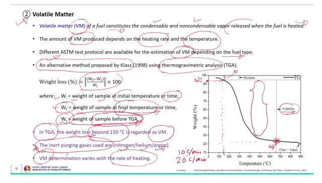
So, the next in the list of approximate analysis is the volatile matter. Volatile matter of a fuel constitutes the condensable and non-condensable vapours released when the fuel is heated and the amount of volatile matter produced is depends on the heating rate and the temperature.
