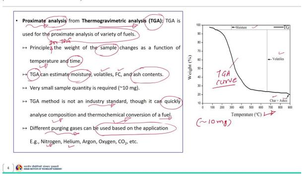
So, now let us discuss about this new method of proximate analysis from the thermogravimetric analysis also known as a TGA. So, this TGA is used for the proximate
