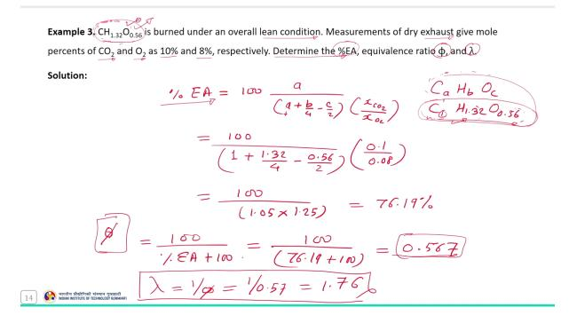
So, in this example the given fuel is burned under an overall lean condition. Measurements of dry exhaust give mole percents of carbon dioxide and oxygen as 10 percent and 8 percent respectively. So, with help of this given data we need to estimate the percentage excess air as well as the equivalence ratio for the given fuel.
