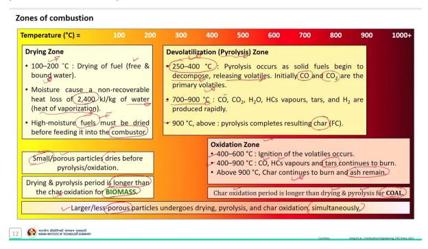
So, the first is the drying zone or we can say the drying stage in which the drying of fuel takes place in the temperature range of 100-200 °C. And during this stage free and the bound moisture or you can say the water release from the fuel. And this moisture it causes a non-recoverable heat loss of 2400 kJ/kg of water, and that is heat of vaporization of water.
