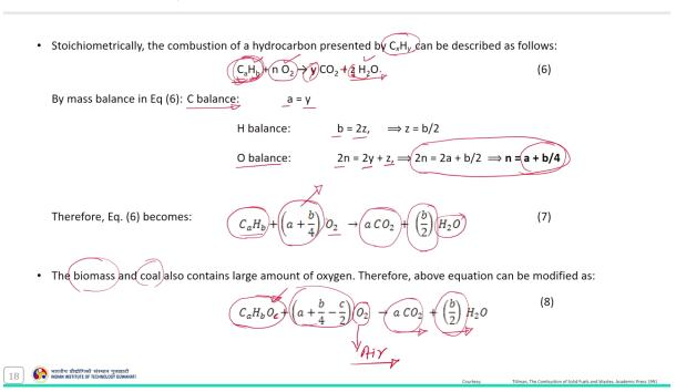
So, normally the combustion of hydrocarbon fuel it represented as C suffix X and H suffix Y and it can be described as follows that is  $C_aH_b$ . And if this hydrocarbon fuel is oxidized with adequate supply of oxygen then it produces y moles of  $CO_2$  plus z mole of water vapor.
