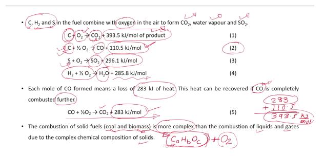
And if you recollect our discussion in one of the module, we discussed about the combustion of the solid fuels. And there we learnt that the elements such as carbon, hydrogen and sulphur in solid fuel only take part into the combustion or you can say the oxidation reaction. And the other element does not take part into the combustion and the oxidation reaction. And when the solid fuel is used for the combustion process, so the carbon, hydrogen and sulfur get oxidized to produce carbon monoxide.
