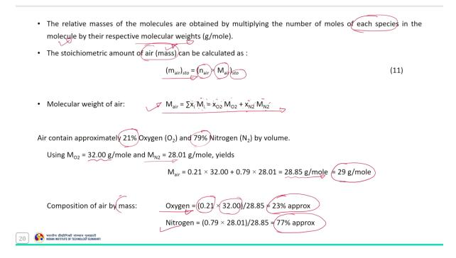
Now, similarly these relative mass of molecules can be obtained by simply multiplying the moles of each species in the molecule by their molecular weights. Say for example, here as the stoichiometric amount of the air need to be calculated that is on the mass basis, so it can be calculated like this.
