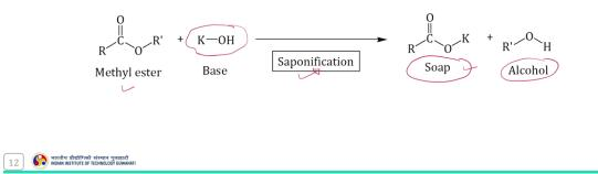
Apart from the catalyst type the catalyst concentration or we normally term it as a catalyst loading is among the most influential parameter which affects the biodiesel yield. Therefore the optimum catalyst concentration should be determined experimentally for attaining the maximum biodiesel yield. And in case if the alkali catalyst concentration exceeds the optimum range then it increases the soap formation and that ultimately lowers the yield of methyl ester.
