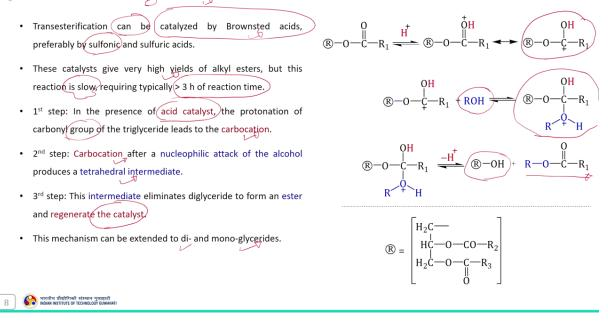
While the mechanism of acid catalyzed transesterification reaction indicates that the transesterification reaction it can be catalyzed by bronsted acids preferably by sulfuric and sulfuric acids. And this catalyst it gives very high yield of alkyl ester. But this reaction is relatively slow compared to that of the alkali catalyst transesterification reaction, and required typically more than 3 hours of the reaction time to complete the transesterification process.
