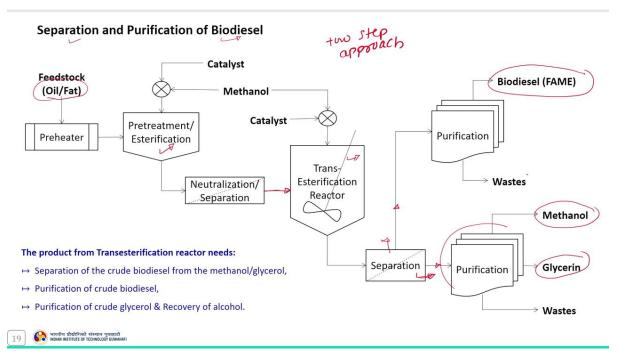
So, the next important topic is the separation and the purification of the prepared biodiesel. So, this schematic here it represent the process arrangement of biodiesel production using two-step approach which includes acid catalyze pre-esterification followed by the base catalyze transesterification reaction to convert the FFA and triacylglycerol into esters.
