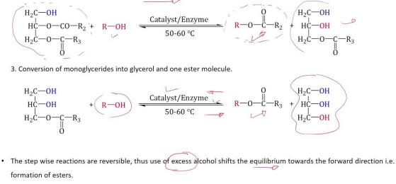
• In presence of excess alcohol, the foreword reaction is pseudo 1<sup>st</sup> order and the reverse reaction is 2<sup>nd</sup> order.
