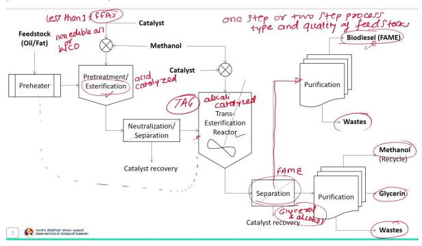
This schematic here it represent the process arrangement of biodiesel synthesis from various oily feedstock materials and also includes the process selection for the biodiesel synthesis. So, this biodiesel production can be carried out as a one step or two step processes depending on the type and quality of feedstock.
