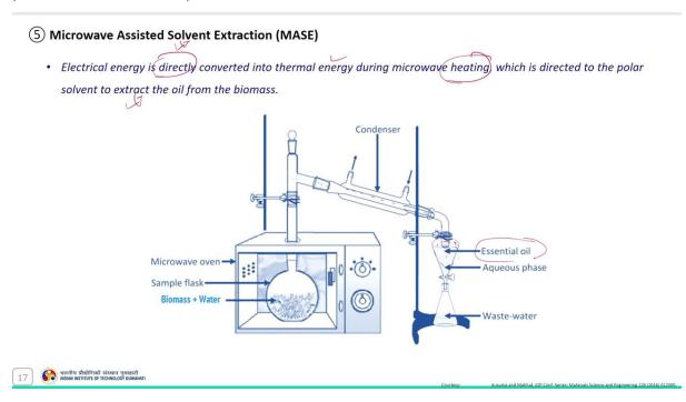
Another important technique which is used for the extraction of oil includes the microwave assisted solvent extraction. So, in this process electrical energy is directly converted into the thermal energy during the microwave heating and which is directed to the polar solvent to extract the oil from the biomass matrix. The solvent along with the extracted components are condensed and allowed to separate here to form aqueous phase and oily phase.
