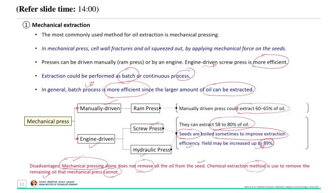
And the most commonly used method for the oil extraction is mechanical pressing. In mechanical pressing, cell wall fractures and oil squeeze out by applying mechanical force on the seed samples. Now, if you look at this particular chart here, these mechanical press methods are of two types that is manually driven and engine driven. However, the engine driven screw press method is more efficient in terms of oil extraction.
