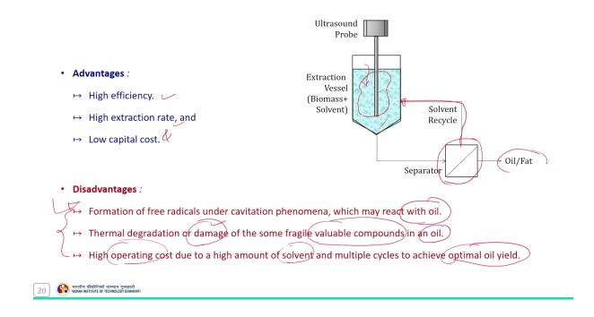
The advantage of this technique includes high efficiency, high extraction rate and low capital cost. However, the free radicals formed during this cavitation phenomenon may react with the oil and that is the major limitation of this process. Similarly the thermal degradation or damage of the some fragile valuable compounds in oil may occur because of these high shock waves, high operating cost due to the high amount of solvent and the multiple cycles to achieve the optimal oil yield.
