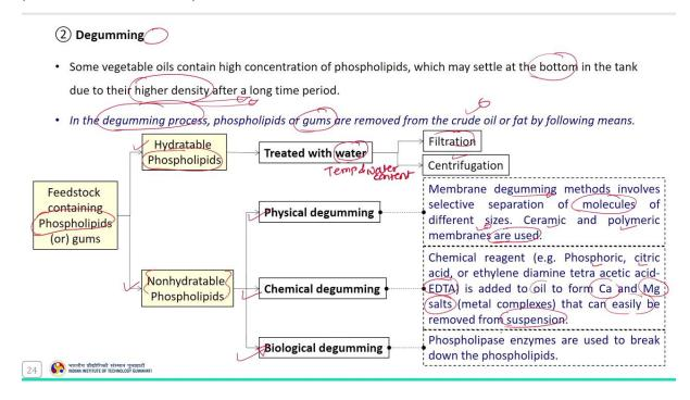
Another important pre-treatment technique is a degumming. Because some feedstock may contain phospholipids which may settle at the bottom in the tank due to their high density.
