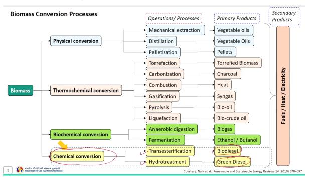
Among these different biomass conversion processes so far we covered thermochemical conversion and the biochemical conversion processes. However, in this module the main focus is on the chemical conversion process that is if you can see here in this chart. So, in this module, we will discuss about the different chemical conversion processes that are transesterification and hydro treatment to produce biodiesel and green diesel as a biofuel.
