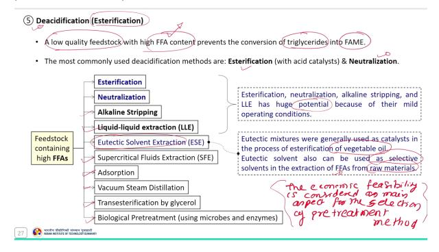
Next is deacidification or esterification. Deacidification normally performs with low quality feedstock with high FFA content. Because this high FFA content in the oily feedstock prevents the conversion of triglycerides into fame. And the most commonly used deacidification methods are esterification and neutralization.
