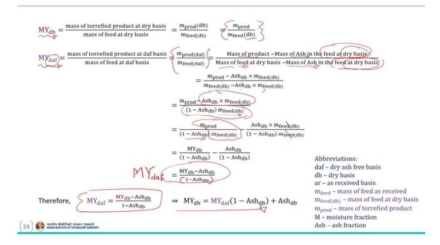
Similarly, these particular terms can be correlated with the mass yield on dry ash free basis. As we represented this equation in the form of mass of product by the mass of feed on dry basis here. Similarly, the mass yield on dry ash free basis can be represented in this form and this equation can be expanded in this particular way here. Because mass of
