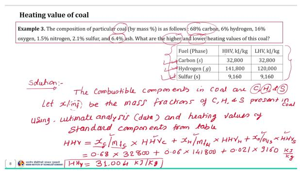
So, the next example it is also in the similar line. So, here we have to calculate the high reading value of the coal sample that is solid fuel. So, for the calculation of this high reading value of this given fuel the composition of the coal sample is given here. So, with the help of this composition we need to estimate the high reading value of the coal. So, let us try to solve this another example on the similar concept.
