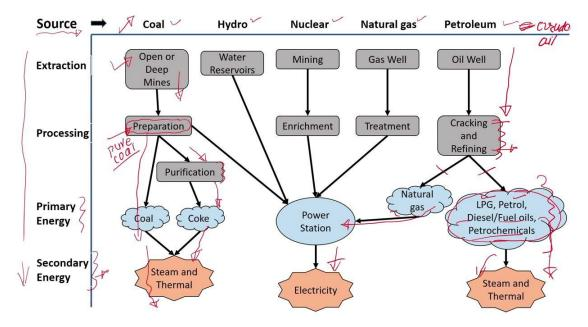
So, let us discuss about this concept in more detail by using this schematic. So, in this case if you see here on the top different sources are named like coal, hydro, nuclear, natural gas and petroleum. On the other side if you can see here these are the different modes of transformation or you can say the conversion to produce first the primary energy source from this raw source and then convert this primary energy source into a secondary energy resources.
