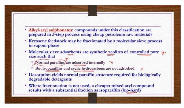
These molecular sieves are nothing but the absorbents which are synthetic zeolites having controlled pore size they are having several applications. But what they do they adsorb internally the normal paraffins which are required for you know for this process that is a good one. But they do not absorb isoparaffins and then cyclic hydrocarbons.
