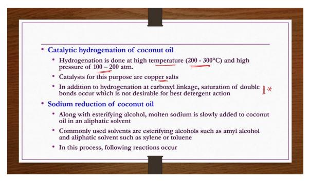
To these fatty alcohols then you do the required reaction with the NaOH and then additives addition etc. if you do you get the detergents. At the end of the reaction batch is
