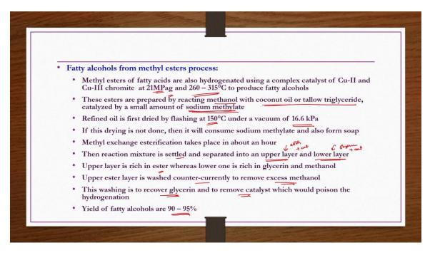
So this is about a fatty alcohols production by the Jiggler processor and then applications of such fatty alcohols. Now we try to see the process how to get the fatty alcohols from methyl esters. Fatty alcohols from methyl esters process. Here methyl esters of fatty acids are also hydrogenated using a complex catalyst of Cu2 and Cu3 chromate at 21 mega Pascal gauge 260 to 315 degrees centigrade to produce fatty alcohols.
