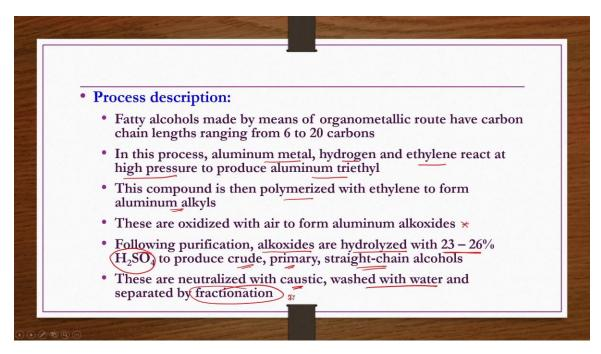
Description of the process is presented here once again. Fatty alcohols made by means of organometallic route have carbon chain lines ranging from 6 to 20 carbons. In this process aluminum metal, hydrogen and ethylene react at high pressure to produce
