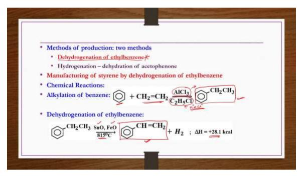
Then methods of production, 2 methods are there, dehydrogenation of ethylene and then hydrogenation of dehydration of acetophenone. However, we discussed this particular method in detail. First, we produce the ethyl benzene in the first step and then in the second step we do the dehydrogenation of ethyl benzene to get the styrene.
