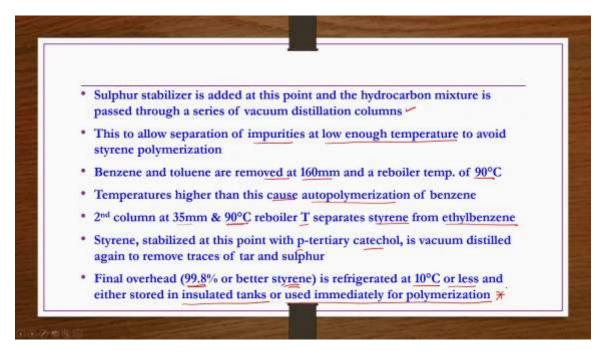
Sulphur stabilizer is added at this point and the hydrocarbon mixture is passed through a series of vacuum distillation columns.
