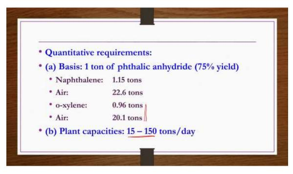
Quantitative requirements, 1 ton of ppphthalic anhydride 75 percent yield. If you are using naphthalene then 1.15 tons and then air, 22.6 tons required. If you are using ortho xylene then 0.96 tons required, air 20.1 tons required. So, requirement of the raw materials is slightly less if you are using xylene in comparison with naphthalene and air. Plant capacities 15 to 150 tons per day.
