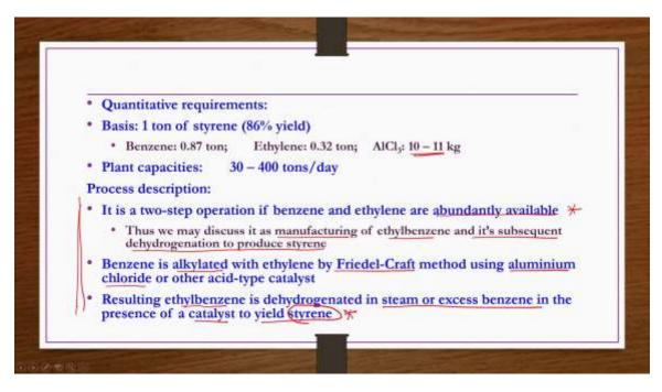
Quantitative requirements, if you want to produce 1 ton of styrene with 86 percent yield, benzene 0.87 tons required, ethylene 0.32 tons required, aluminum chloride 10 to 11 kgs.
