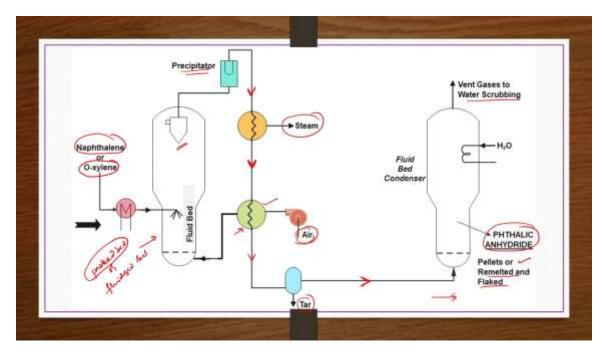
This is the flowchart provided here. So, whether you take naphthalene or ortho xylene or mixture of it, what you have to do? You have to preheat it and then melt it and then that melted mixture of the reactants or individual reactants are fed to a reactor.
