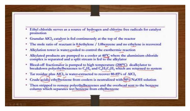
Ethyl chloride serves as a source of hydrogen and chlorine free radicals for catalyst promotion. Granular aluminum chloride catalyst is fed continuously at the top of the reactor.
