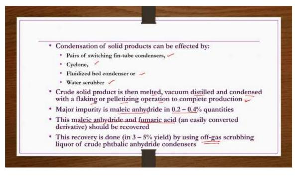
Condensation of solid products can be affected by pairs of switching fin-tube condensers or cyclones or fluidized bed condensers or water scrubbers any of them can be used or all of them may be used in general. Crude solid product is then melted vacuum distilled and condensed with a flaking or pelletizing operation to complete the production of a dry pellets of phthalic anhydride or flakes of phthalic anhydride.
