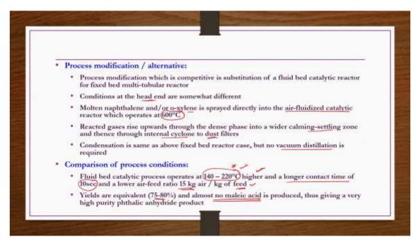
Process modifications and alternatives as already mentioned in place of fixed bed reactors we can also have fluid bed reactors as well. So, let us say if you use the fluid bed reactors then conditions at the head end are somewhat different. Molten naphthalene or ortho xylene is spread directly into the air fluidized catalytic reactor which operates at 600 degrees centigrade slightly higher temperature than the case of packed bed reactors.
