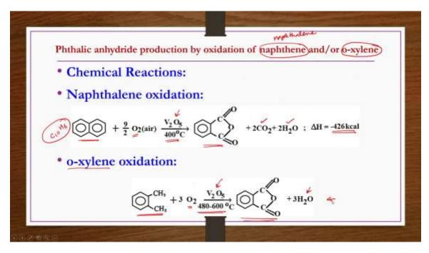
Now, we discussed the production of pphthalic anhydride using the naphthalene raw material that is if you do the oxidation of naphthalene, then you can get the pphthalic anhydride or if you do the oxidation of ortho xylene, then also you can get the pphthalic anhydride or you take the mixture of these 2 and do the oxidation of the mixture, then also you get the pphthalic anhydride.
