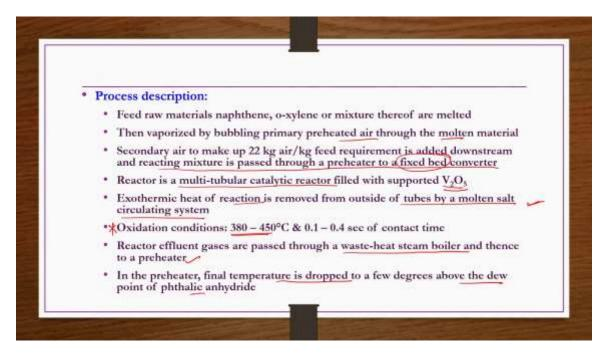
Process description feed raw materials naphthalene, ortho xylene or mixture thereof are melted then vaporized by bubbling primary preheated air through the molten material.
