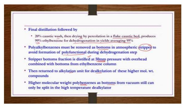
Final distillation followed by 20 percent caustic wash then drying by percolation in flake caustic bed produces 99 percent pure ethyl benzene for dehydrogenation step in yields averaging 95 percent. Polyalkylbenzene must be removed as bottoms in the atmospheric stripper to avoid formation of poly functional during dehydrogenation step.
