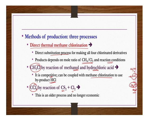
Coming to the methods of production 3 processes are existing. The first one is direct thermal methane chlorination that is you just take methane and then chlorine of appropriate mole ratio as per the product distribution that you wanted to have and then do the thermal reaction. Just heat it at 370 to 400 degrees centigrade depending on the product distribution.
