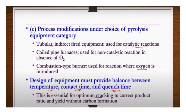
Coming to the process modification and the choice of pyrolysis equipment category, tubular indirect fired equipment are used for catalytic reactions. Coiled pipe furnaces are
