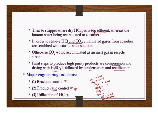
Then to stripper where dry HCl gas is top effluent whereas the bottom water being recirculated to the absorber. In order to remove HCl and CO2, chlorinated gases from absorber are scrubbed with caustic soda solution otherwise CO2 would accumulated as an inert gas in a recycle stream. Final steps to produce high purity products are compression and drying with H2SO4 is followed by condensation and rectification.
