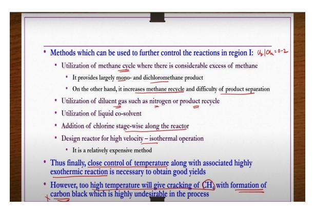
Methods which can be used to further control the reaction in region where Cl2 to CH4 ratio is between 0 to 2. So, what are they utilization of methane cycle where there is considerable
