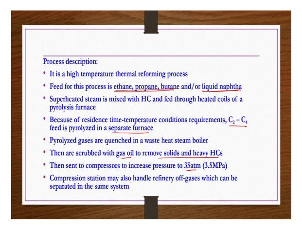
Process description, it is a high temperature thermal reforming process, feed for this process is ethane, propane, butane or liquid naphtha as well. So, depending on the feed, your temperature and then reaction time are going to change that is the reason depending on the feed for these feed you have separate furnace and then for these feed you have separate furnace.
