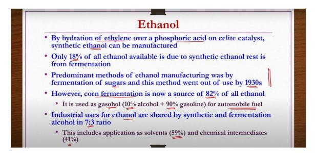
Ethanol it can be obtained by the hydration of ethylene over a phosphoric acid on celite catalyst. So since we are producing this ethanol by the synthetic process so this is known
