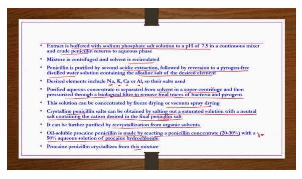
Whereas the extract is buffered with sodium phosphate salt solution to a pH of 7.5 in a continuous mixer and crude penciling returns to aqueous phase.
