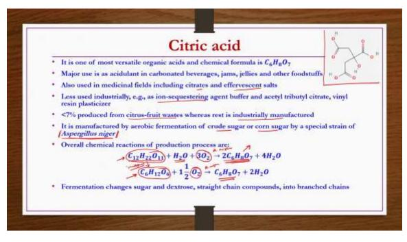
We start with citric acid. Citric acid it is one of the most versatile organic acids and chemical formula is  $C_6H_8O_7$  it is a branched organic chemical and the structure is shown here it is a branched structure here as shown here. Major use is as acidulant in carbonated beverages, jams, jellies and other foodstuffs, etc. It is also used in medicinal fields including citrates, effervasins, salts, etc. for those purpose used.
