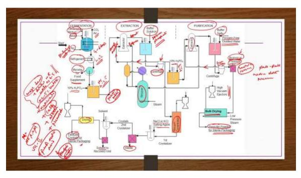
Now, here flowchart for the production of penicillin is shown penicillin in the powder form penicillin in the crystalline form as well. So, here what we have we have a fermenter to which air is being sparse from the bottom because it is also forming by aerobic fermentation process, whatever the fermentation medium mold, etc. they are added to the fermenter reactor and then air is being supplied from the bottom.
