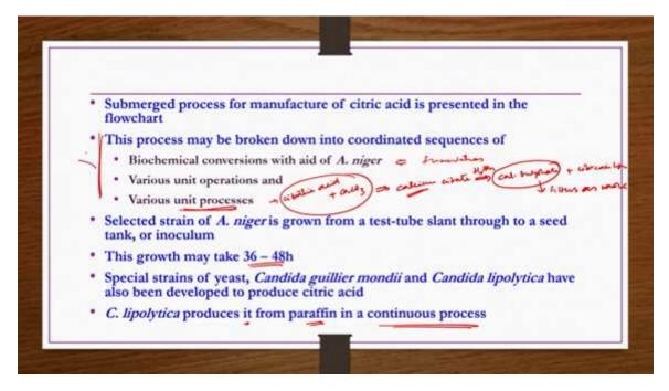
Submerged process for manufacture of citric acid is presented in the flow chart. This process may be broken down into coordinated sequence of obviously biochemical conversion with aid of Aspergillus niger, A niger.
